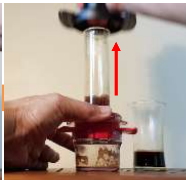
Pull out Piston to bring air into Chamber (air layer helps press water out)
