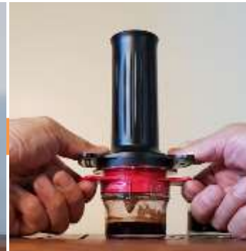
Press Piston down, keep squeezing until water (pressure) fully out of Chamber
